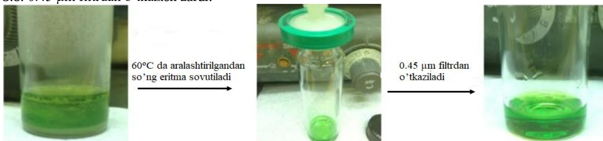
1-rasm. Spin-coating usulida NiOx qatlamini olish ishlatiladigan eritmaning sovutish va filtrlash jarayonidan keyingi holati.
