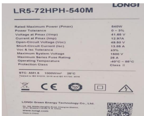
2-rasm. LR5-72 HPH 540M quyosh panelining texnika pasporti
